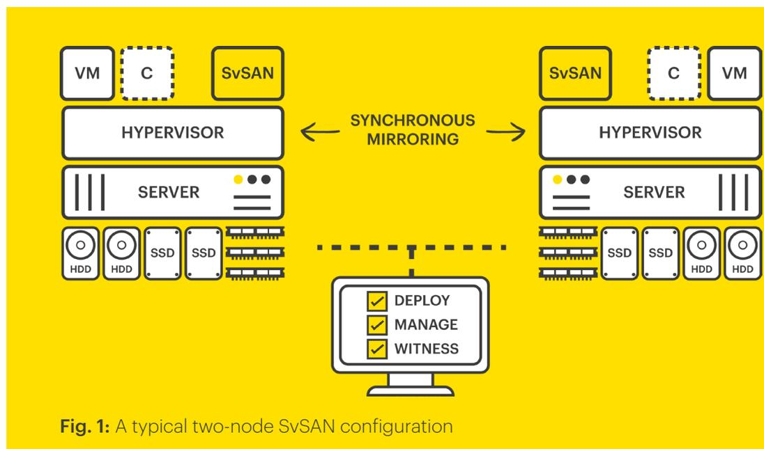
Fig. 1: A typical two-node SvSAN configuration
